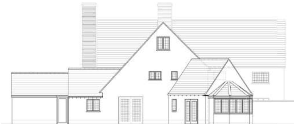
Existing Rear Elevation
