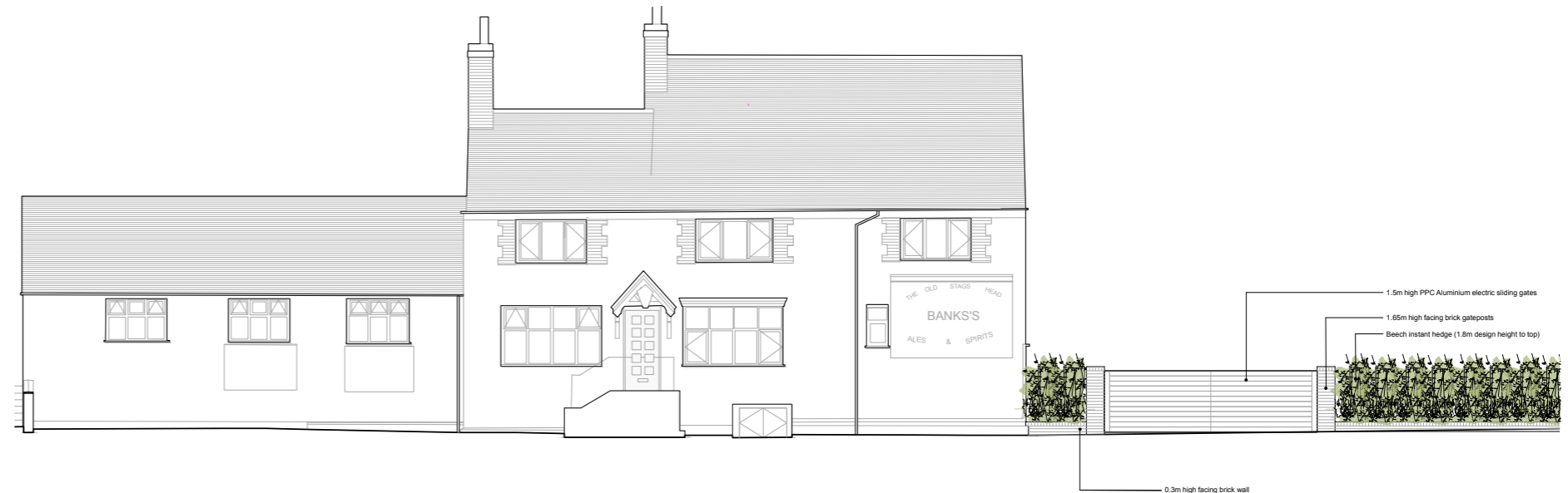
3.5.1 Proposed Front (South West) Elevation showing new boundary treatment to the east
