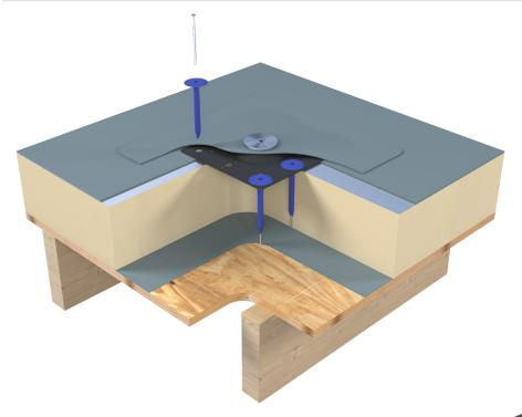
Typical warm roof construction with roofing membrane laid in insulation and utilising thermally broken fixings
