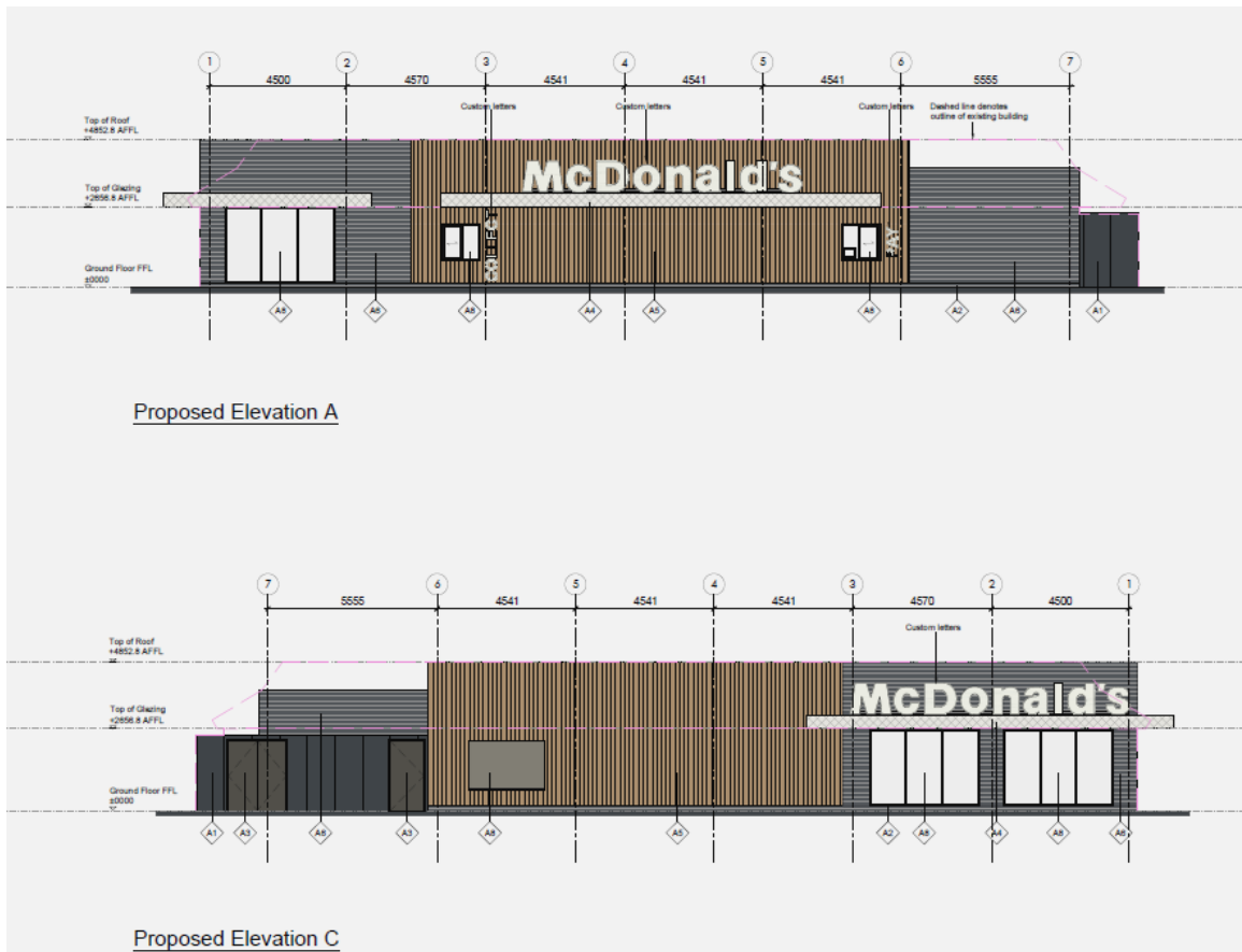
Extract of the proposed elevations with dashed line to show original building
