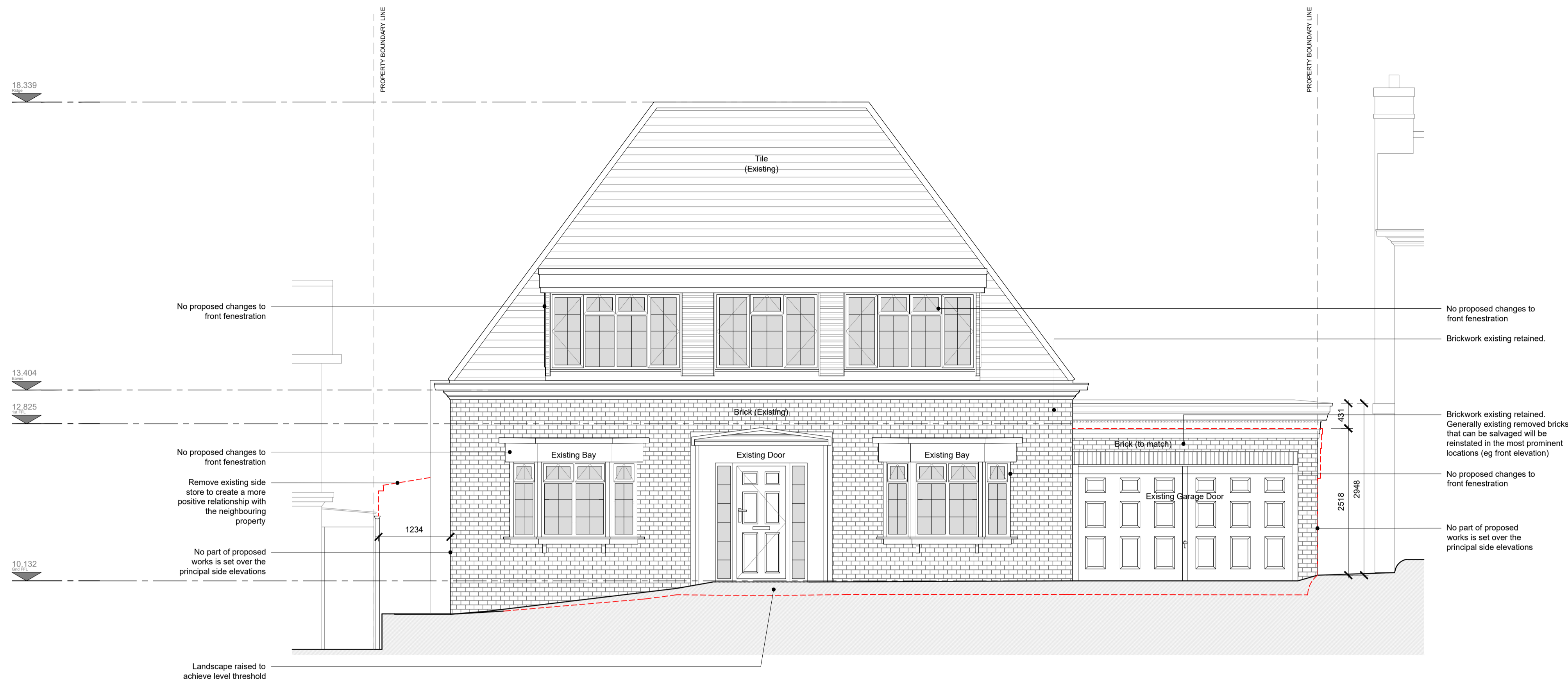
1 Proposed South-East Elevation 1:50 0 0.5 1.0 2.0 3.0 4.0 5.0 Scale in metres
