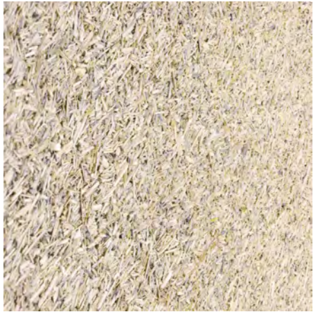
Wood fibre board such as HEMSPAN® Bio Board is a 100% breathable, natural fibre interior construction board product consisting of hemp straw and a mineral binding agent. The pure natural materials, water resistance and breath-ability contribute to a healthy living environment.
