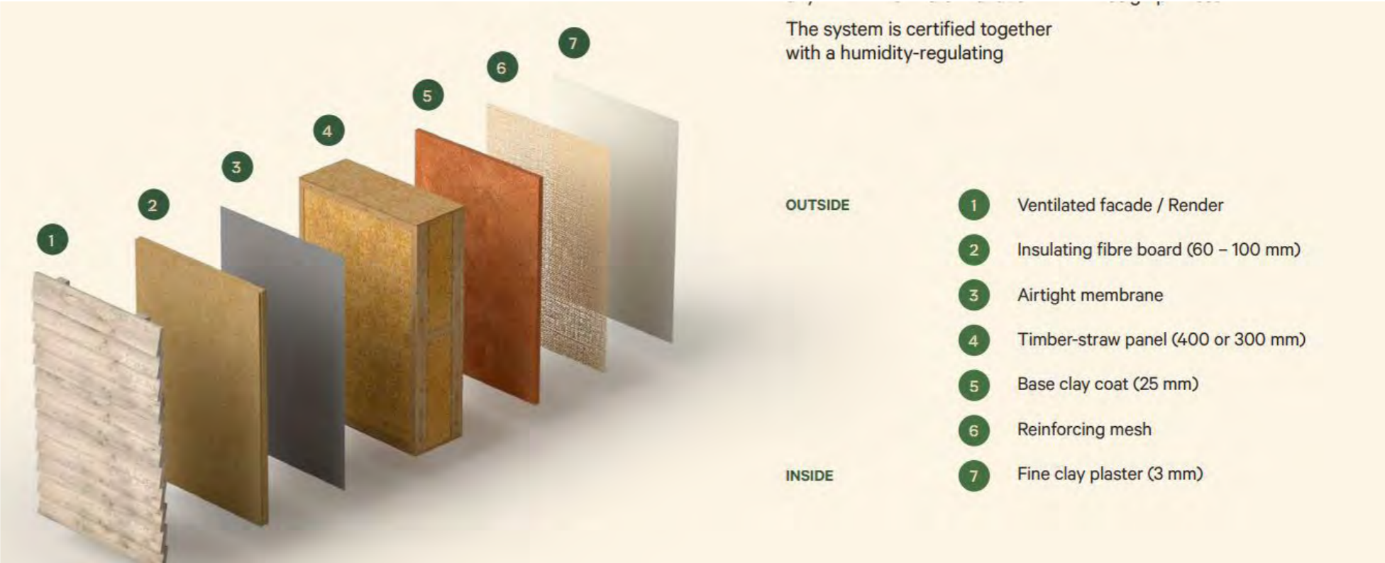
The EcoCocon straw panel innovative wall system is revolutionising construction by making the best of natural materials while ensuring healthy, comfortable, and energy-efficient living at the same time.
