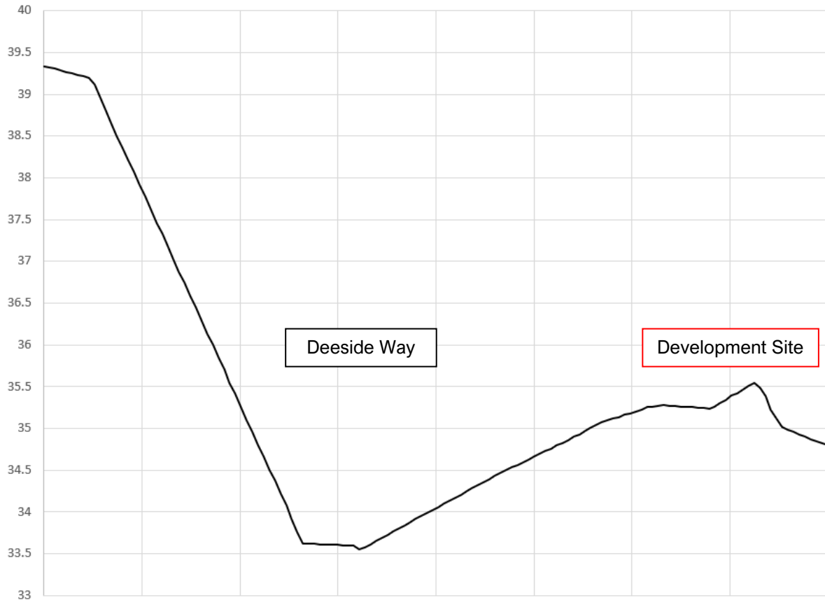
Figure 2.8 Section A-A, through Deeside Way and the adjacent field at the western end of the development site
