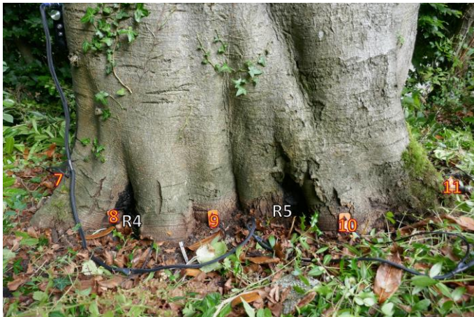
Pl. 6 - PiCUS MPs 7 - 11 at 5cm agl shown in red. Resistograph drill points R4 & R5
