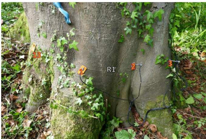
Pl. 4 - PicCUS MPs 13 & 1-3 at 5cm agl shown in red. Resistograph drill point R1
