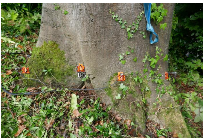
Pl. 7 - PiCUS MPs 11-13 & 1 at 5cm agl shown in red. Resistograph drill point R6
