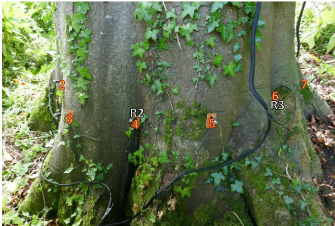
Pl. 5 - PiCUS MPs 2-7 at 5cm agl shown in red. Resistograph drill points R2 & R3
