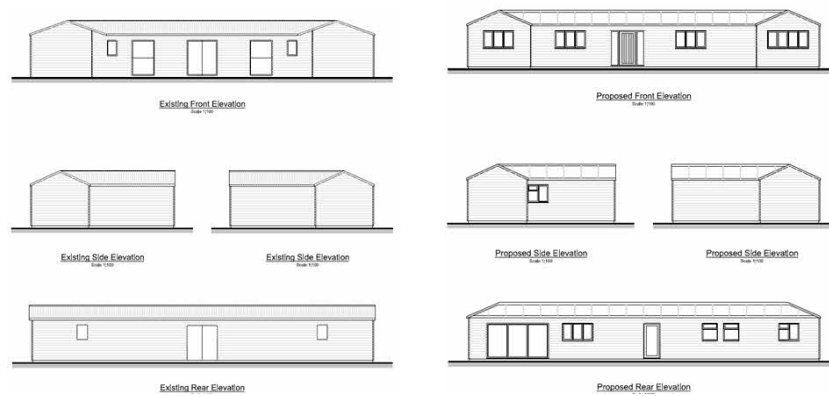
Existing Elevations Proposed Elevations
