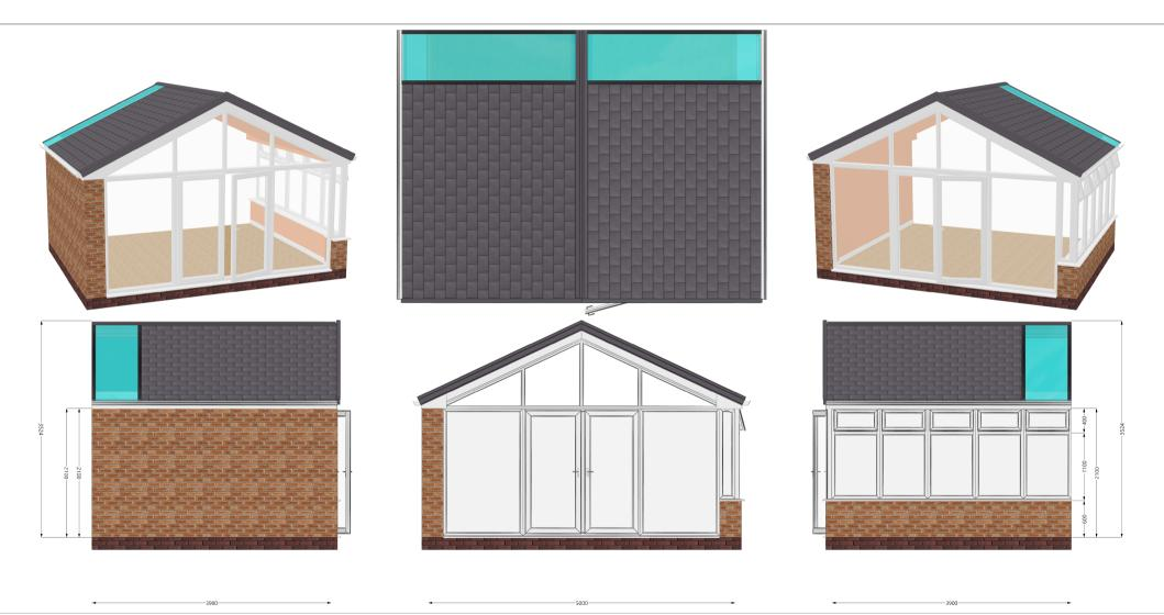
Span: 5000 mm Projection: 3900 mm Colour: White Throughout Glazing: Carbon Grey
