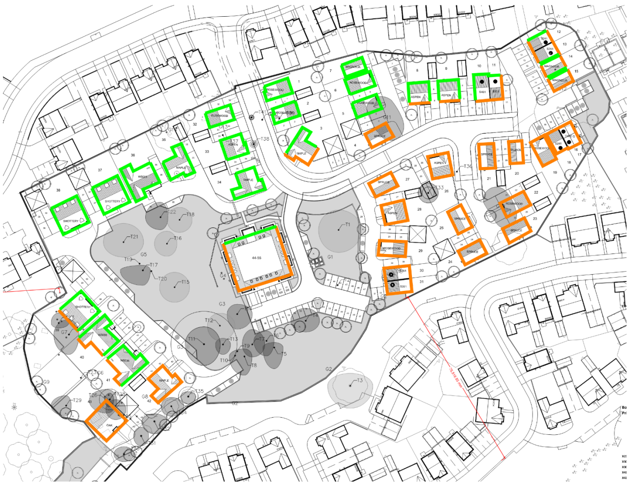
Figure 3 Minimum sound insulation performance required for glazing and the suggested background mechanical ventilation strategy for each building façade (please read together with table 5 above)
