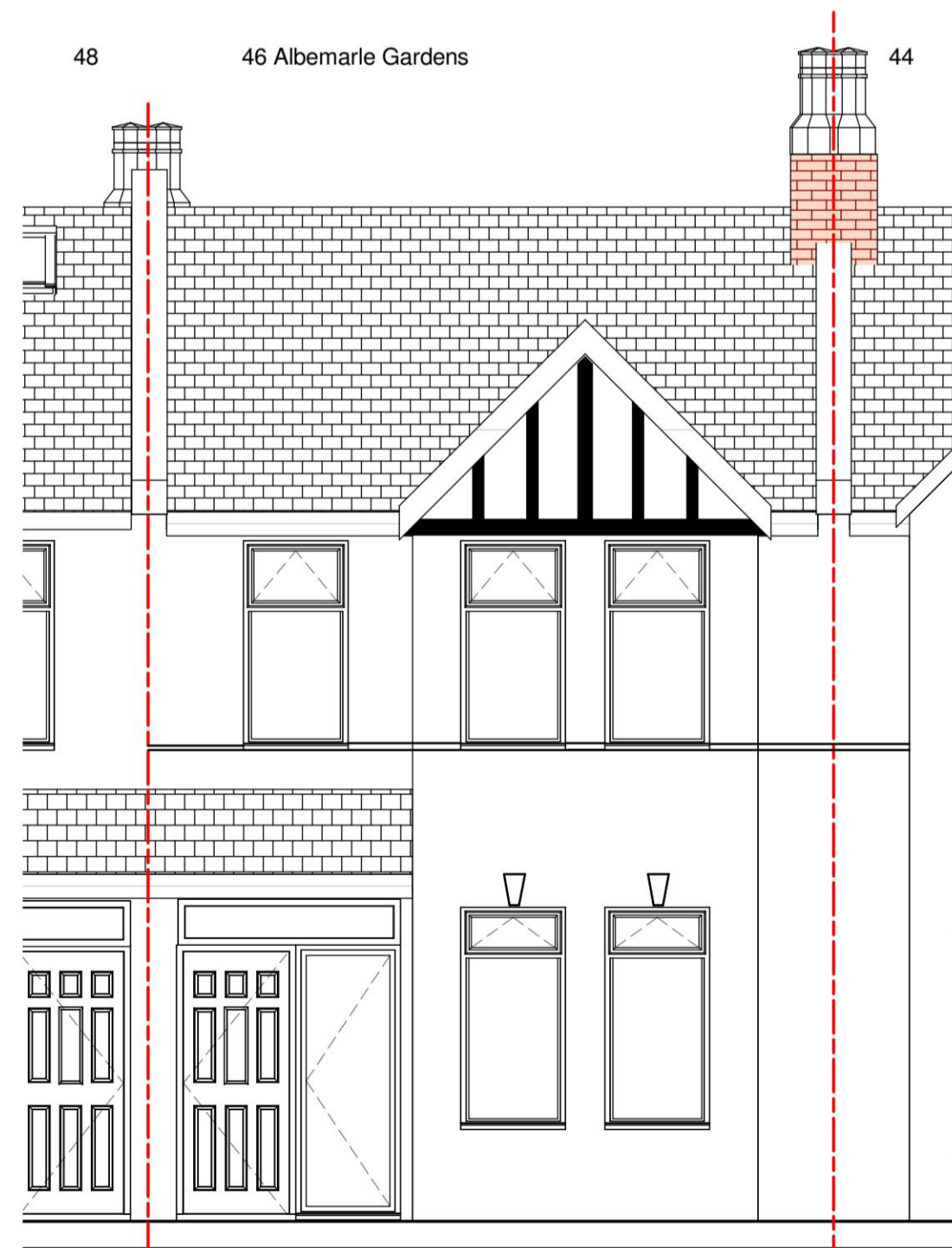
4 Proposed Front Elevation 1 : 50
