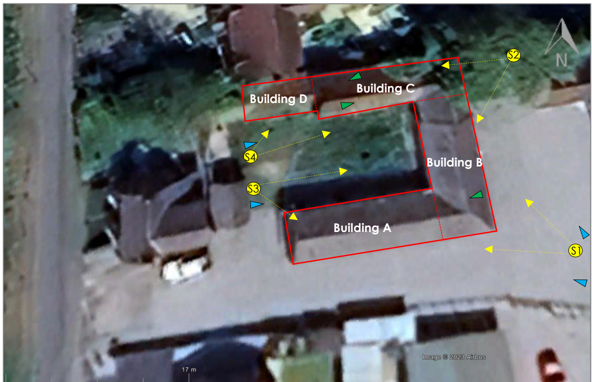
Figure 2. Surveyor and IR/Thermal Camera Locations. Yellow circles = surveyor positions with field of view denoted by yellow dashed arrow / blue triangles = cameras locations for both surveys / green triangles = camera locations for survey two only.
