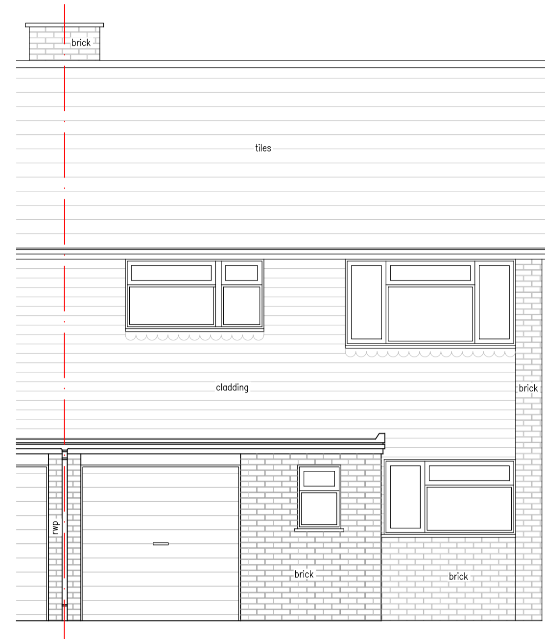
existing front elevation 1:50
