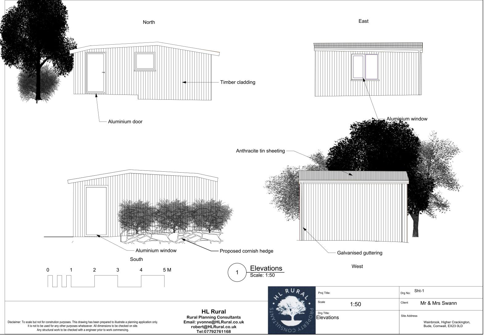
Disclaimer: To scale but not for constrution purposes. This drawing has been prepared to illustrate a planning application only. It is not to be used for any other purposes whatsoever. All dimensions to be checked on site.
