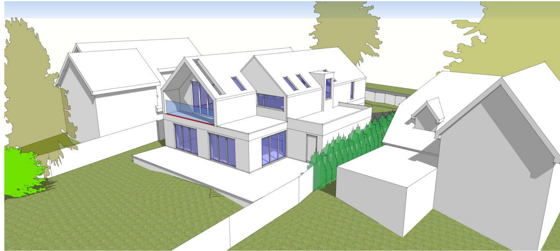
Rear view showing first floor gable and flat roof to living area
