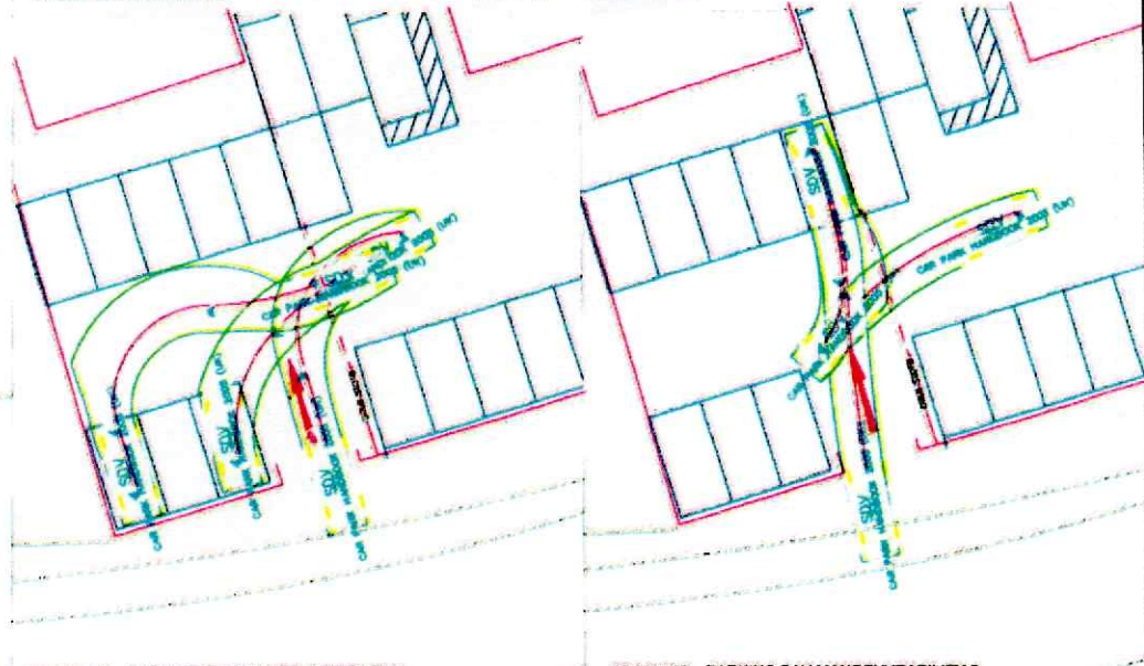
TRACKING - PARKING BAY MANOEUVRABILITY 1
