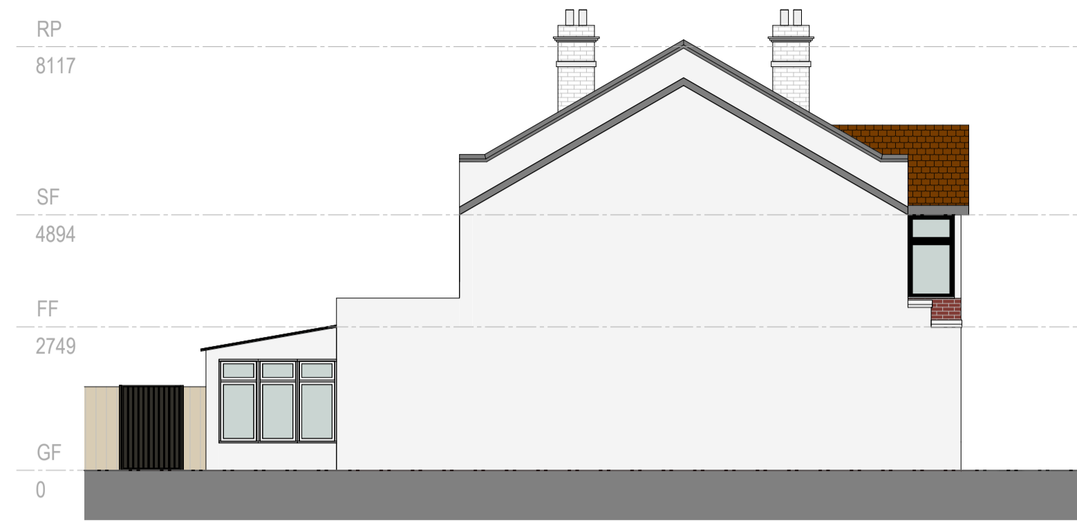
West Side Elevation - Existing 1:100
