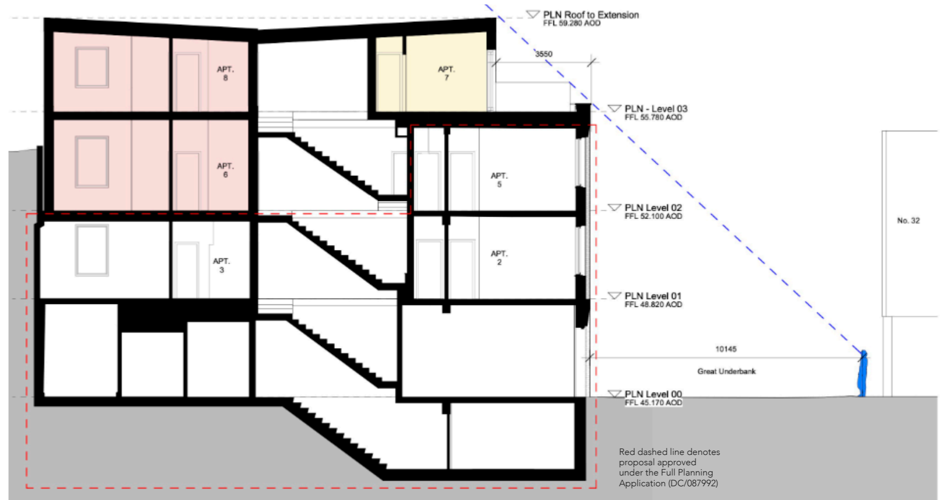
Sight-line Section Diagram and Proposed Vertical Extension Set-back
