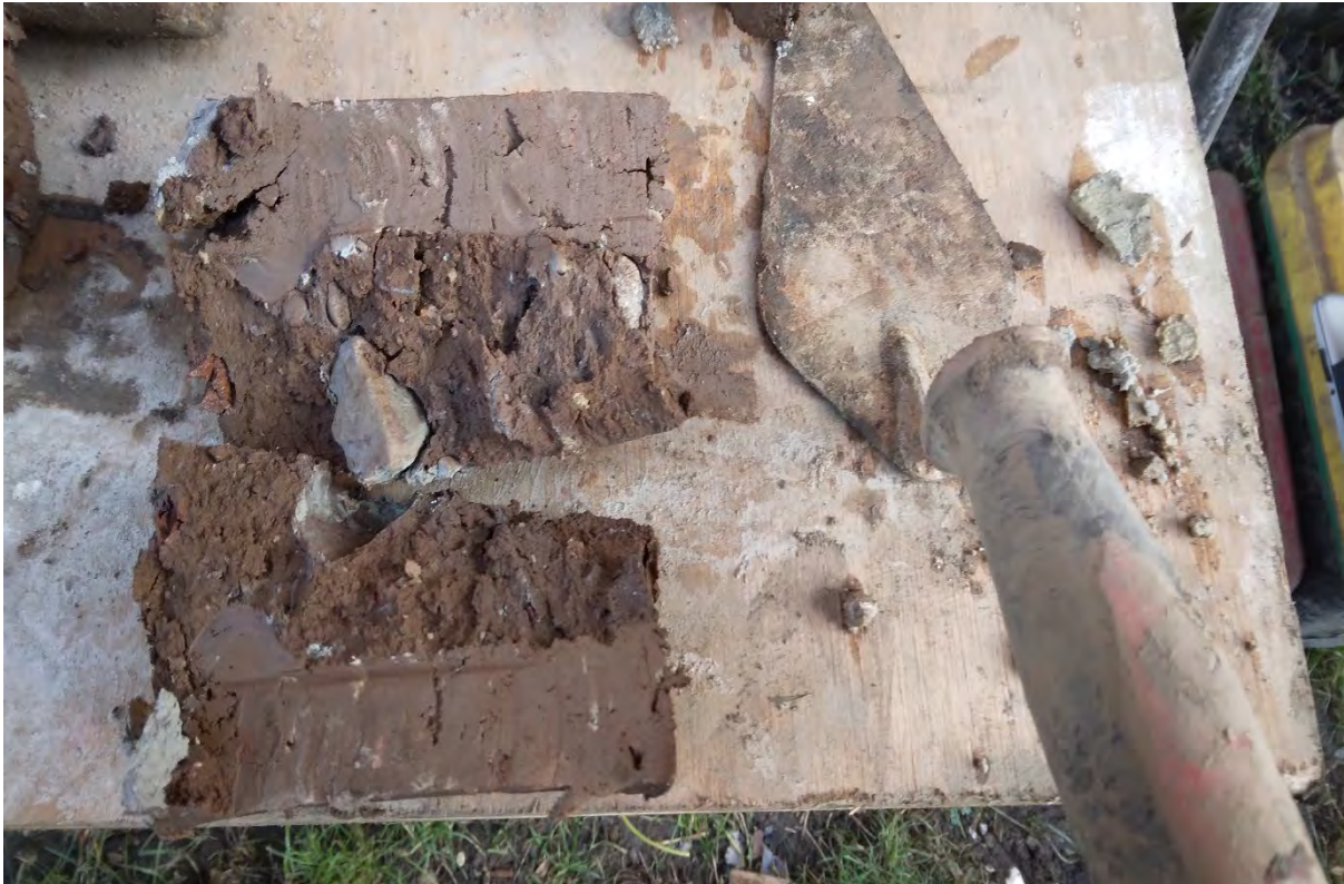
Detailed view of split core recovery from BH03 (1.6m to 1.8m bgl).
