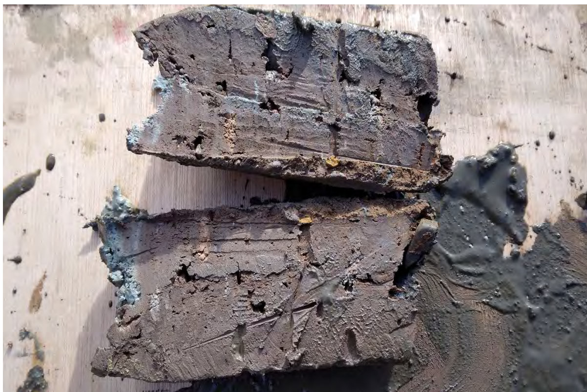
View of split for recovery of natural soils from BH01 (2.0m to 2.2m bgl).
