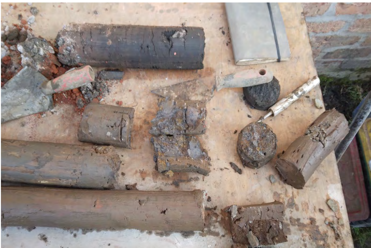
View of overall core recovery from natural soils at BH03.
