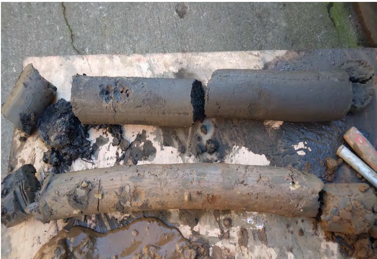
View of core recovery from BH04 (2.0m to 3.0m bgl).
