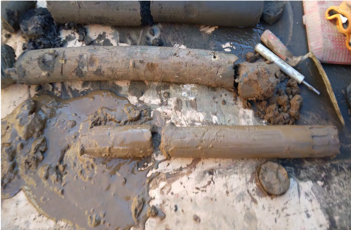
View of initial core recovery from BH04 (note water strike).
