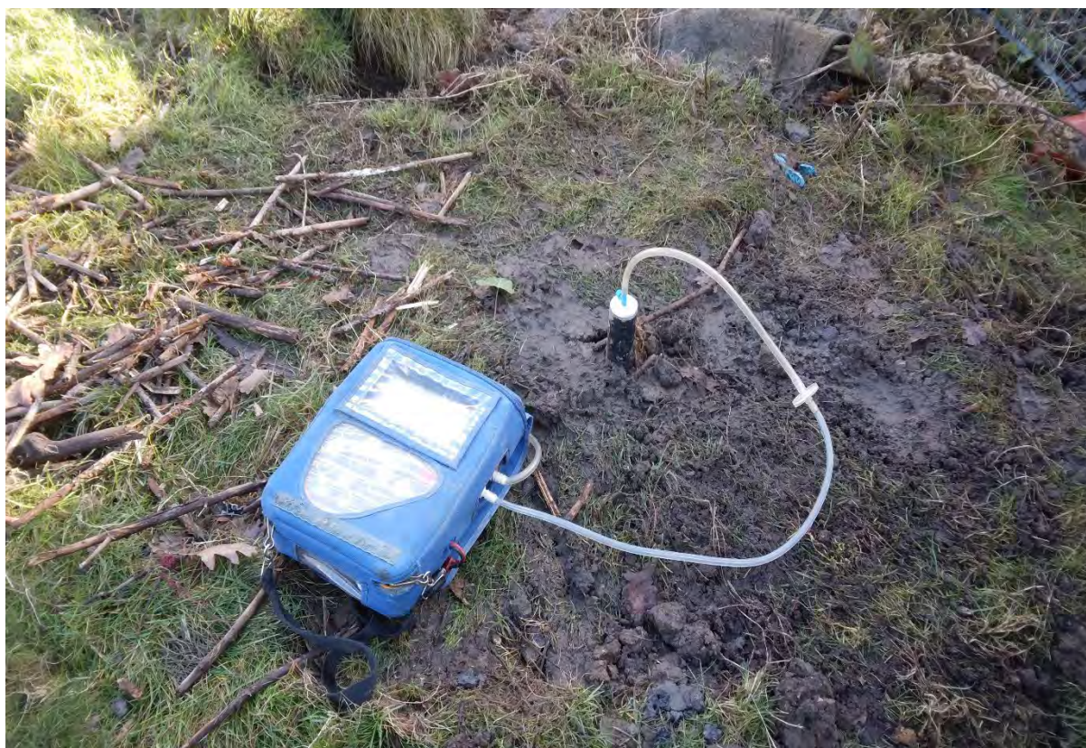
Detailed view of ground gas monitoring at BH01.
