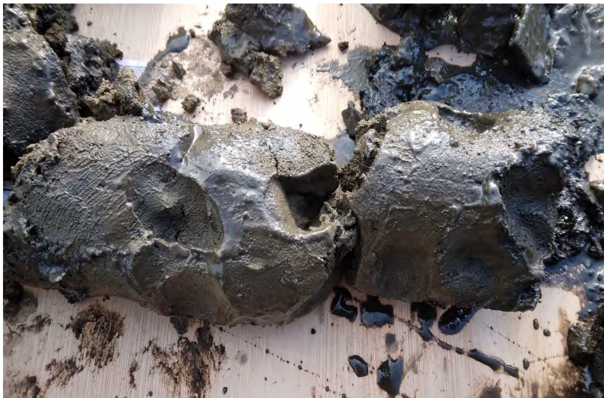
View of initial (soft) recovered natural soils at BH01 (1.0m to 1.3m bgl).
