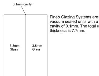
vacuum sealed units with a cavity of 0.1mm. The total unit thickness is 7.7mm.
