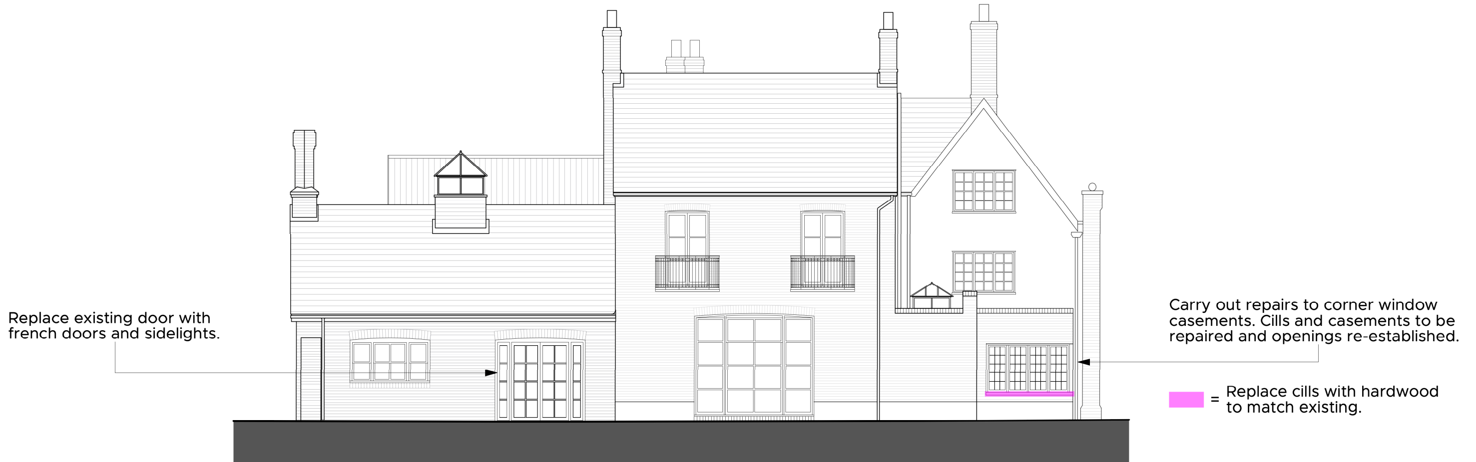
Proposed West Elevation Scale: 1:100
