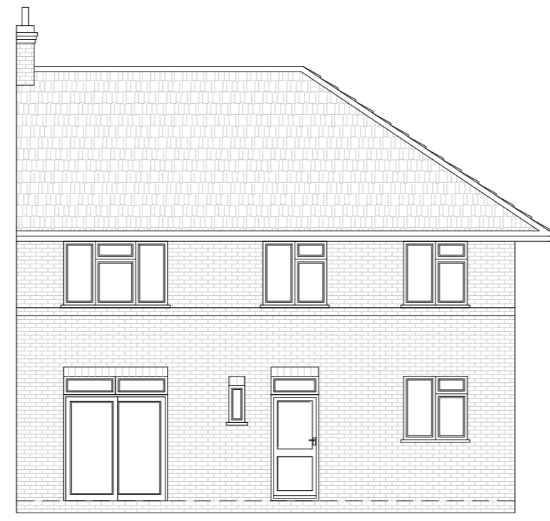
PROPOSED REAR ELEVATION 1:100
