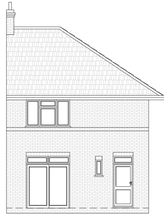
EXISTING REAR ELEVATION 1:100
