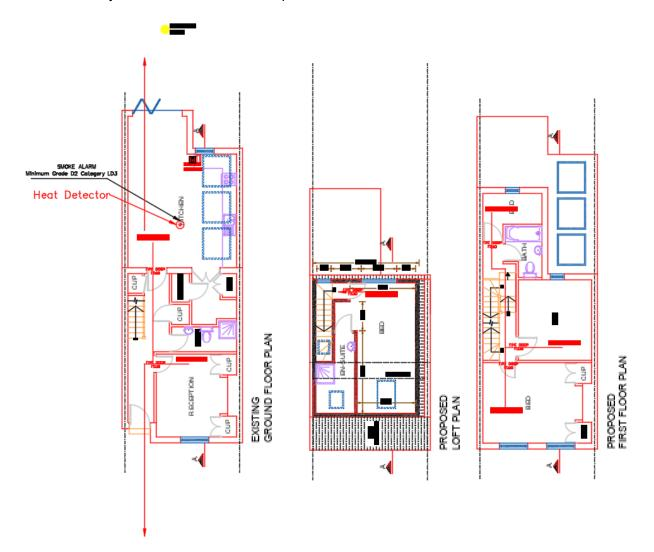
compliant fire doors between the kitchen and the stairs will be installed. Smoke and carbon monoxide alarm detectors are installed that would follow the current regulations.
