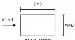
Inwind depth D=15 m Cross wind width B=5 m
