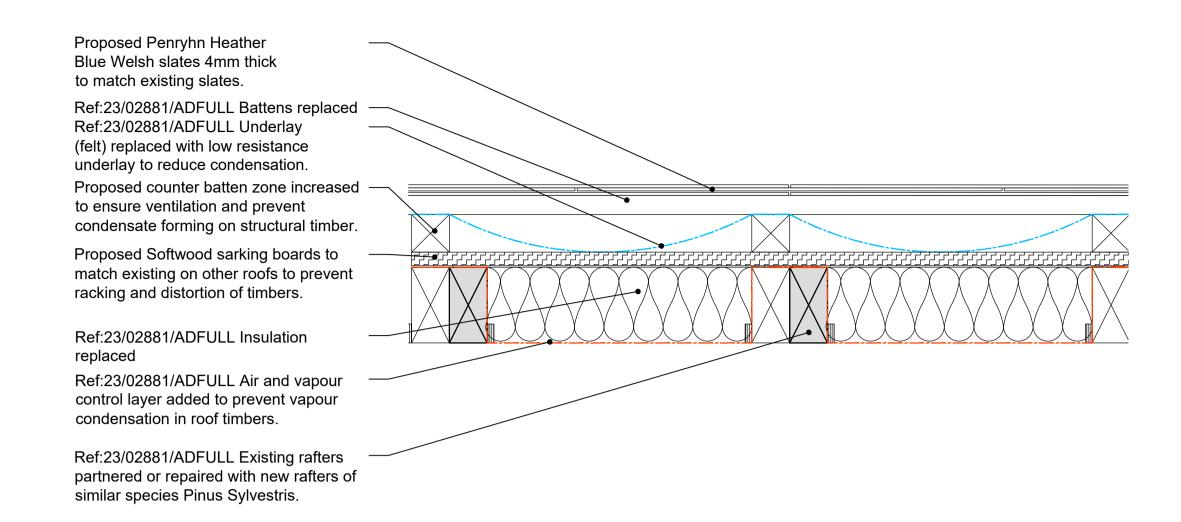
As Proposed typical cross section of upper rafters Scale 1:5 @ A1
