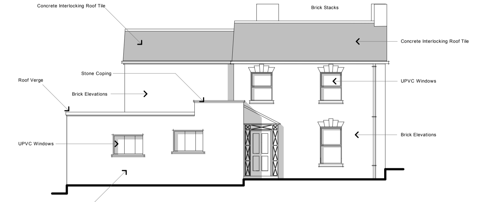
EXISTING FRONT FACING (WEST) ELEVATION
