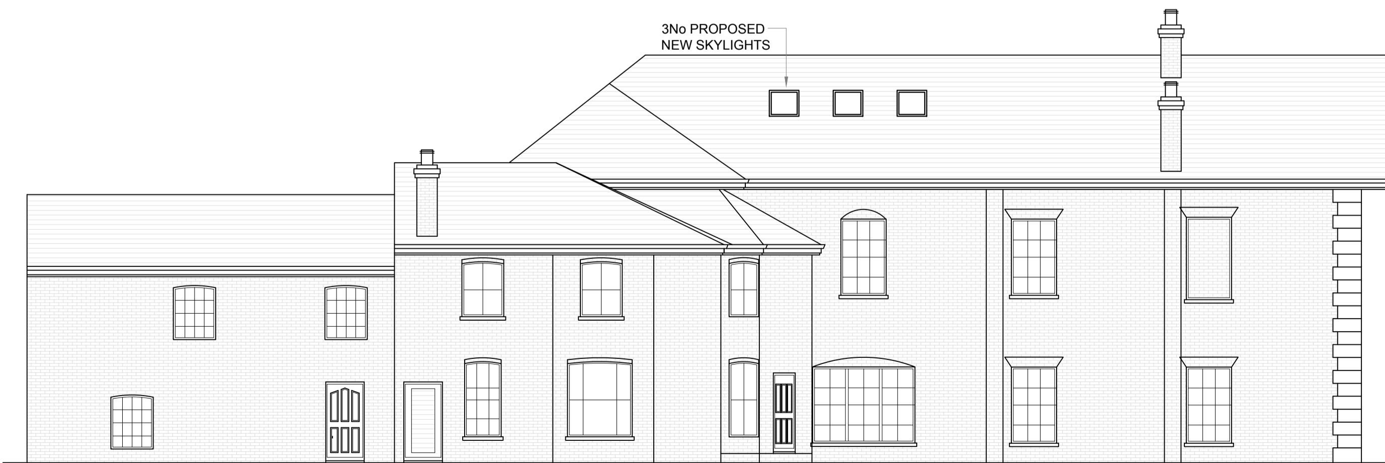
SIDE ELEVATION - PROPOSED SCALE 1:100
