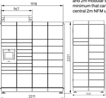
Note: InPost Lockers increase in 0.5m 1m and 2m modular sections up to 12 m with the minimum that can be installed being the central 2m NFM unit.
