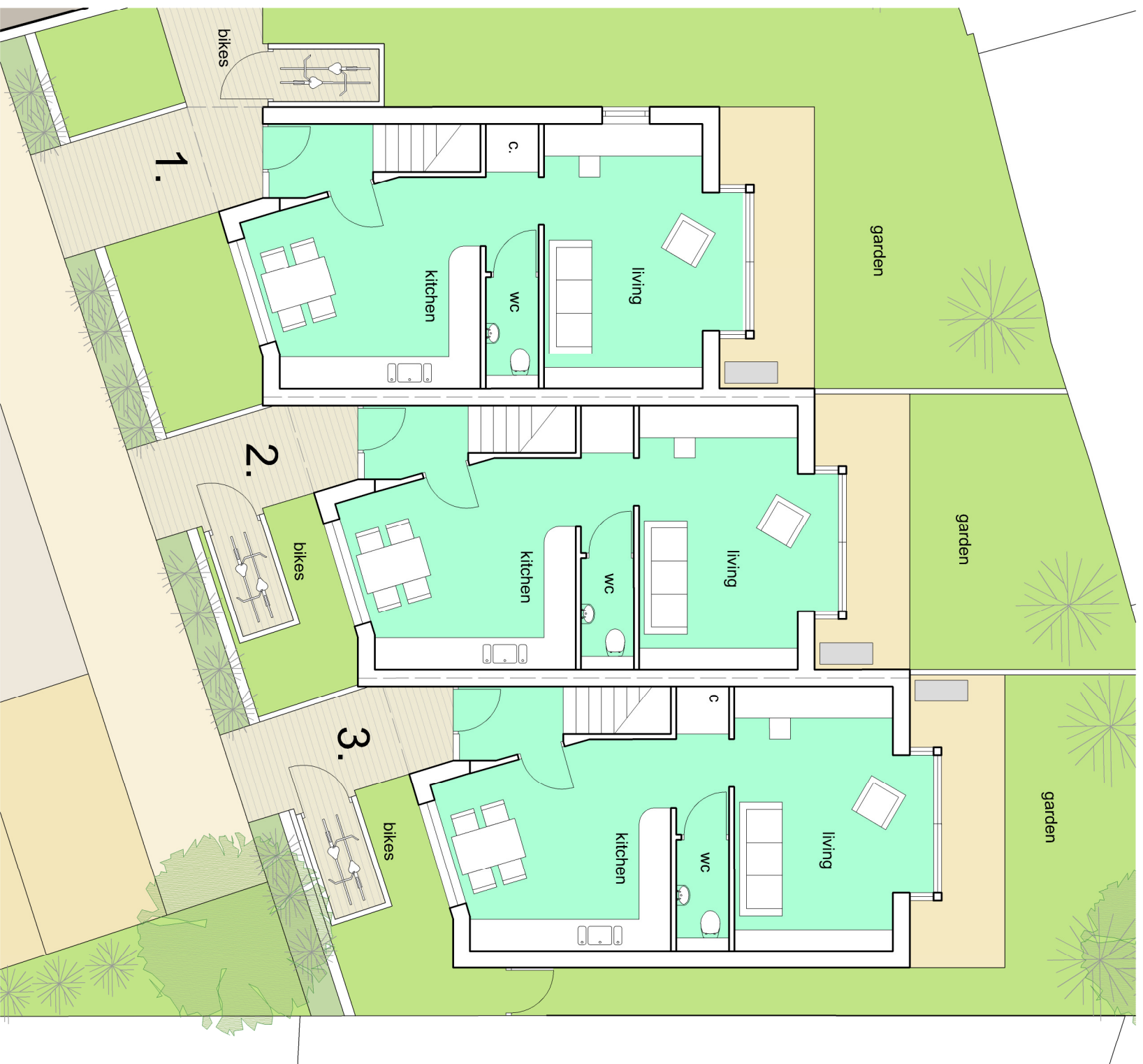
Proposed ground floor plans Scale 1:100 @A3
