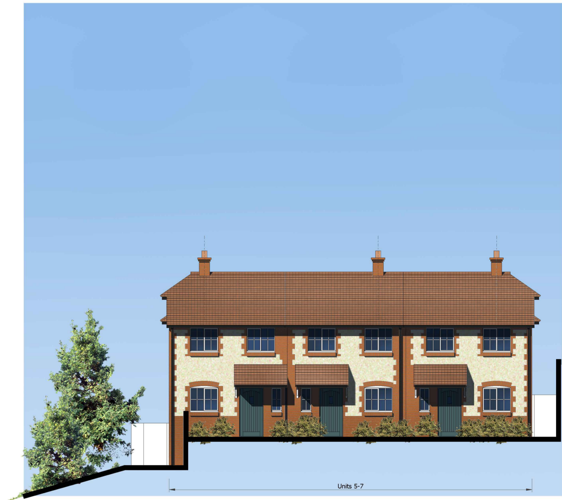
North-West Elevation - materials - roof - plain tiles / walls - face brick and stonework / door + windows - painted timber / rw goods - pvc-u
