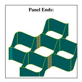
Cellweb Tree Root Protection System: Section diagram example
