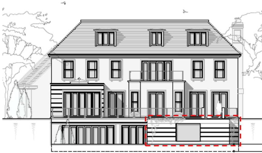
Extract from Proposed Rear Elevation (proposed extension outlined in red dashed line)
