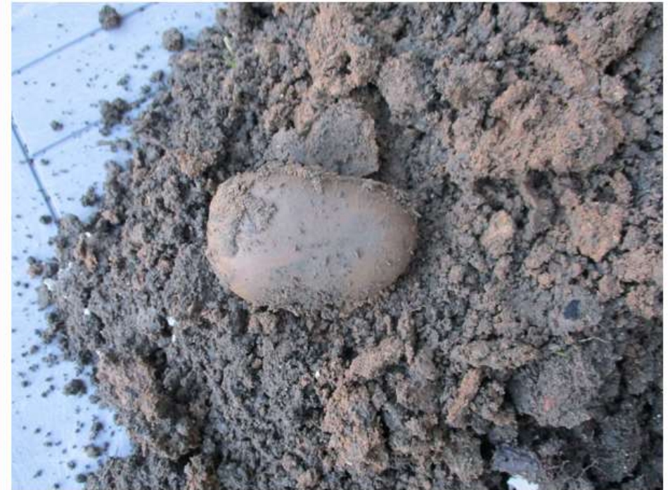
Photo No.2: HP01 pit spoil showing sandy clay, topsoil and rounded gravel inclusions
