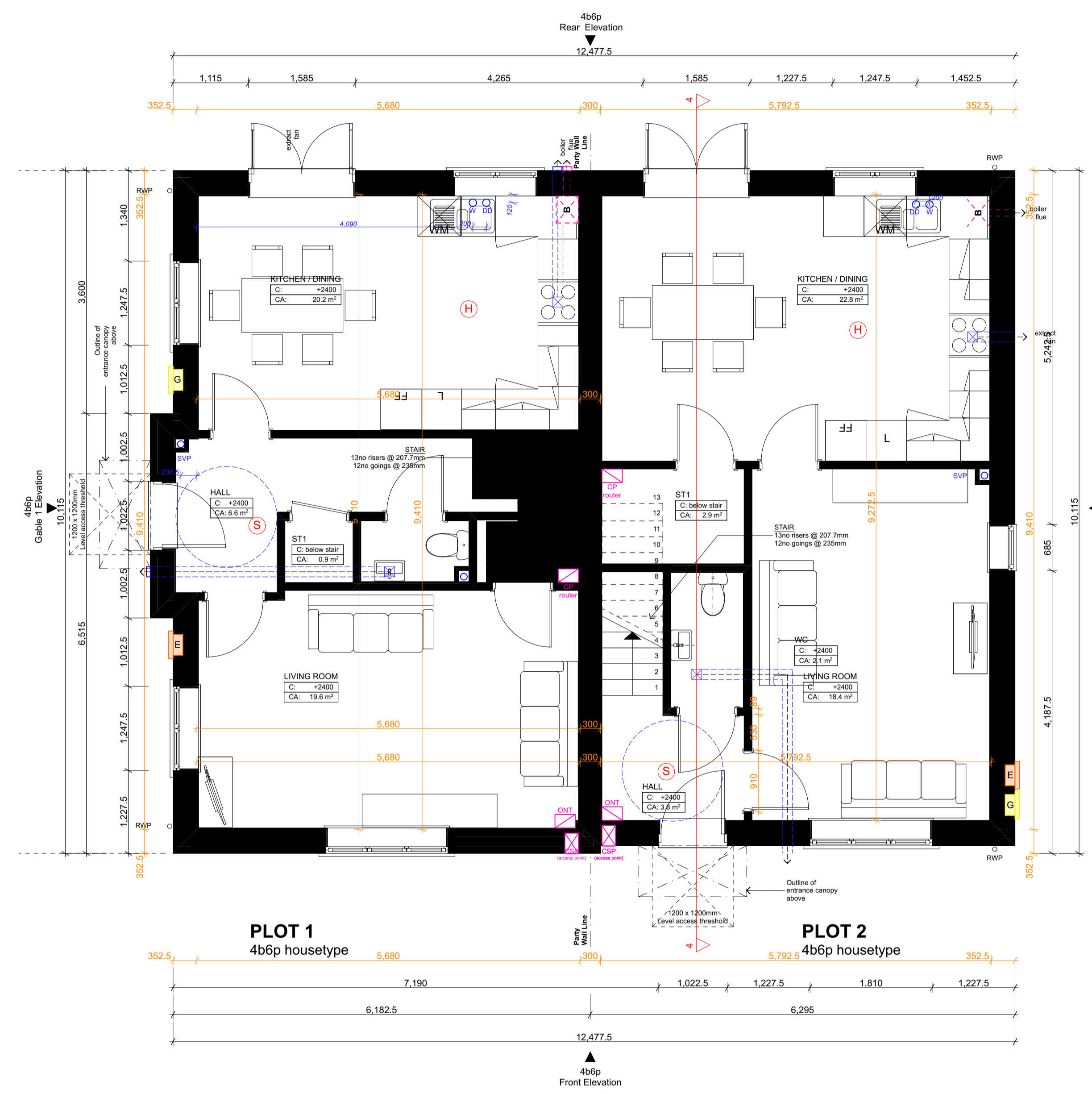
4b6p House type pair - GROUND FLOOR BLOCK PLAN 1:50
