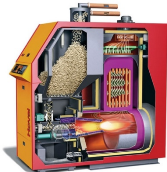
Figure 4: Biomass Boiler diagram
