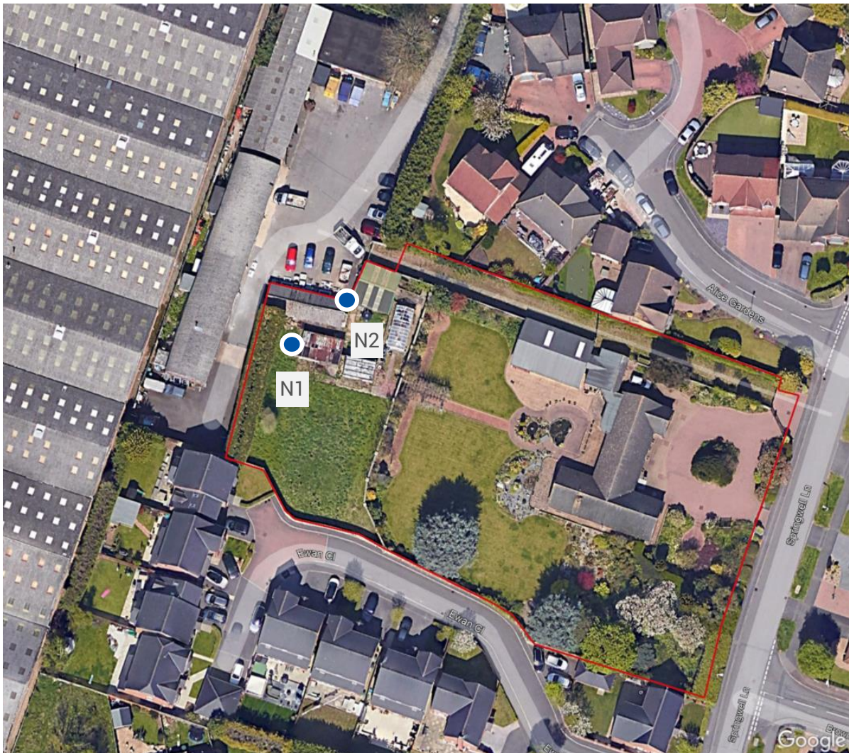
Fig 4.1 Site plan indicating noise measurement positions N1 and N2 Imagery © 2023 Bluesky, Getmapping plc, Infoterra Ltd & Bluesky, Maxar Technologies Map data © 2023 Google
