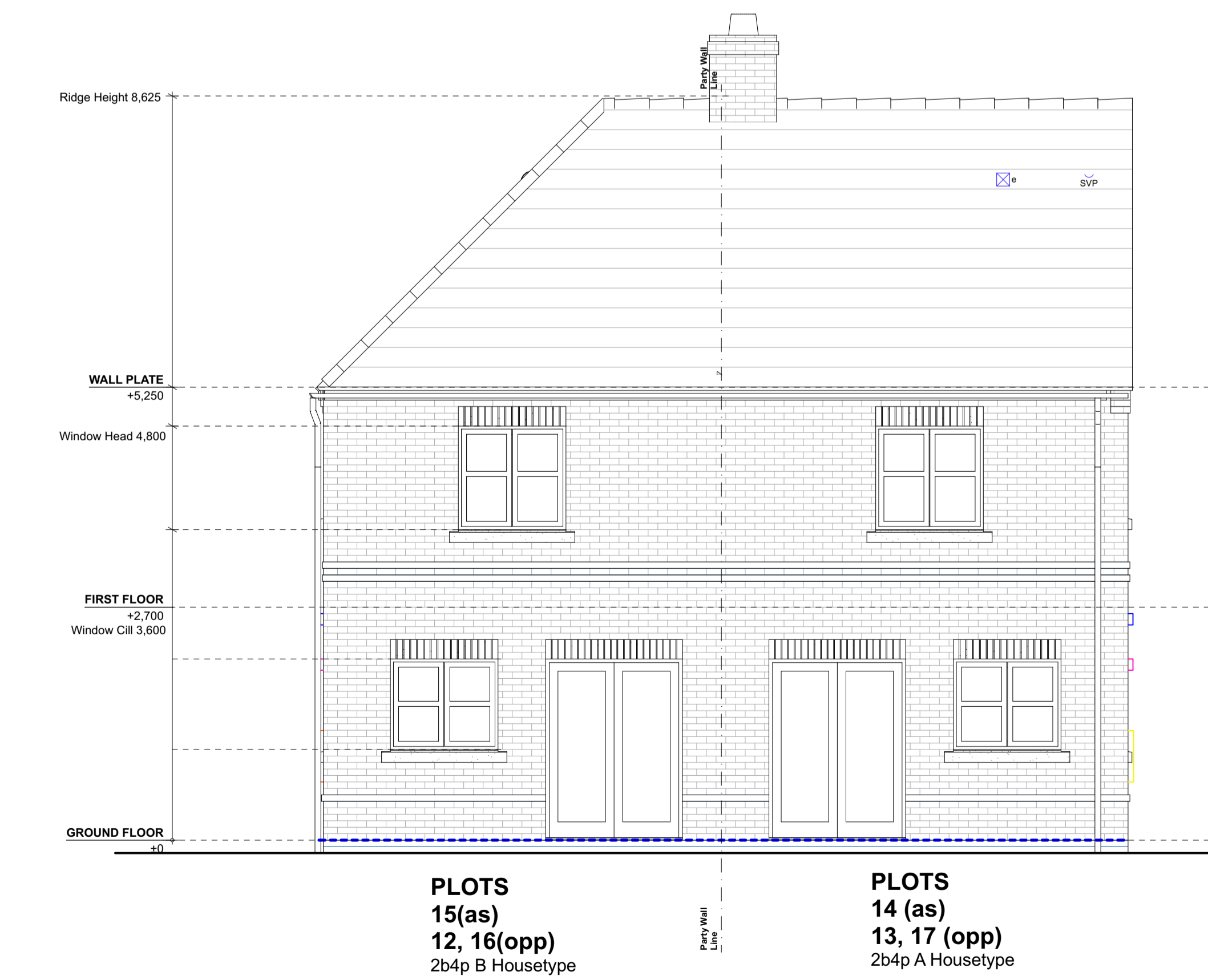
Type AB Rear Elevation 1:50
