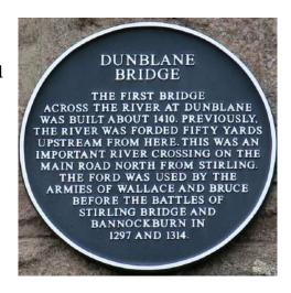
The plaques will be circular, measuring 406mm in diameter. They are cast aluminium and painted black with raised lettering and circular border band in white. They will be installed using an aluminium baseplate, also painted black. The baseplate will use non-ferrous fixings to attach to masonry and a bracket where signposts or railings are being used. The plaque will be mounted on the baseplate using an all-weather adhesive.
