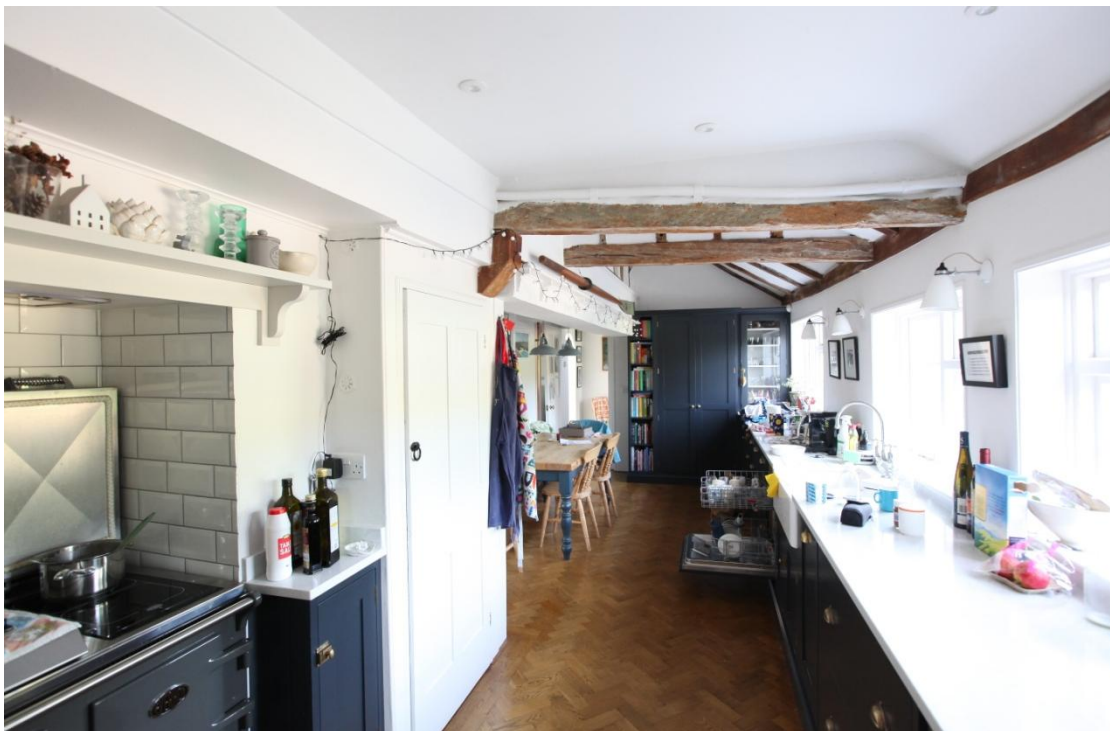
Illus. 10. The interior of the rear lean-to containing the modern kitchen from its south-eastern gable. The space is undivided and heated by an inserted 19 th century chimney in the service cross-wing on the left that probably occupies the position of its original stair.
