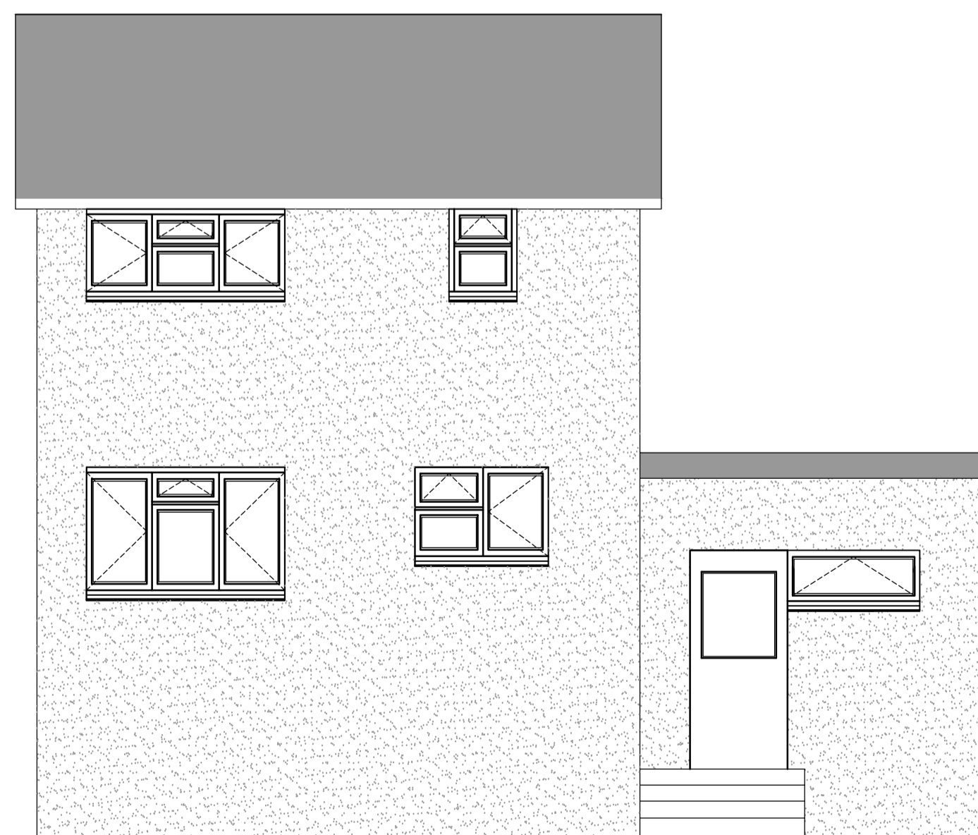
PROPOSED REAR ELEVATION OF No. 19 (NE/NORTH FACING) 1:50
