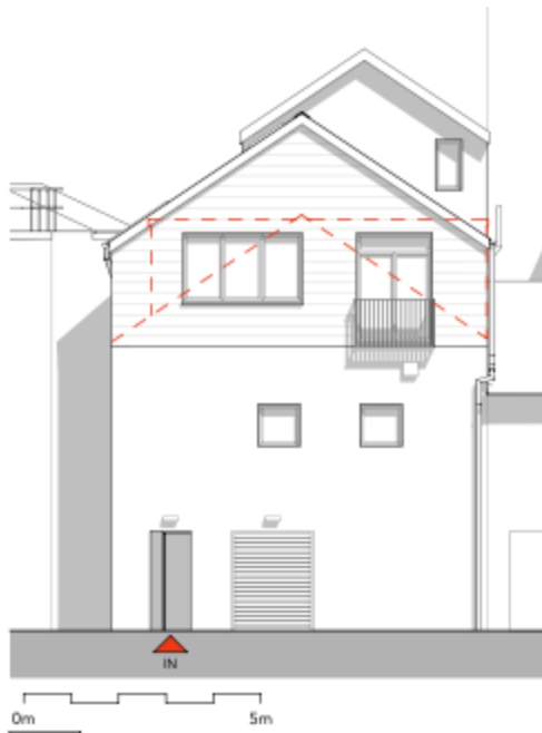
Figure 3: Proposed West Elevation showing roof line to be demolished as broken redlines and LB eaves to left. -drawing no. 023-36 320-01
