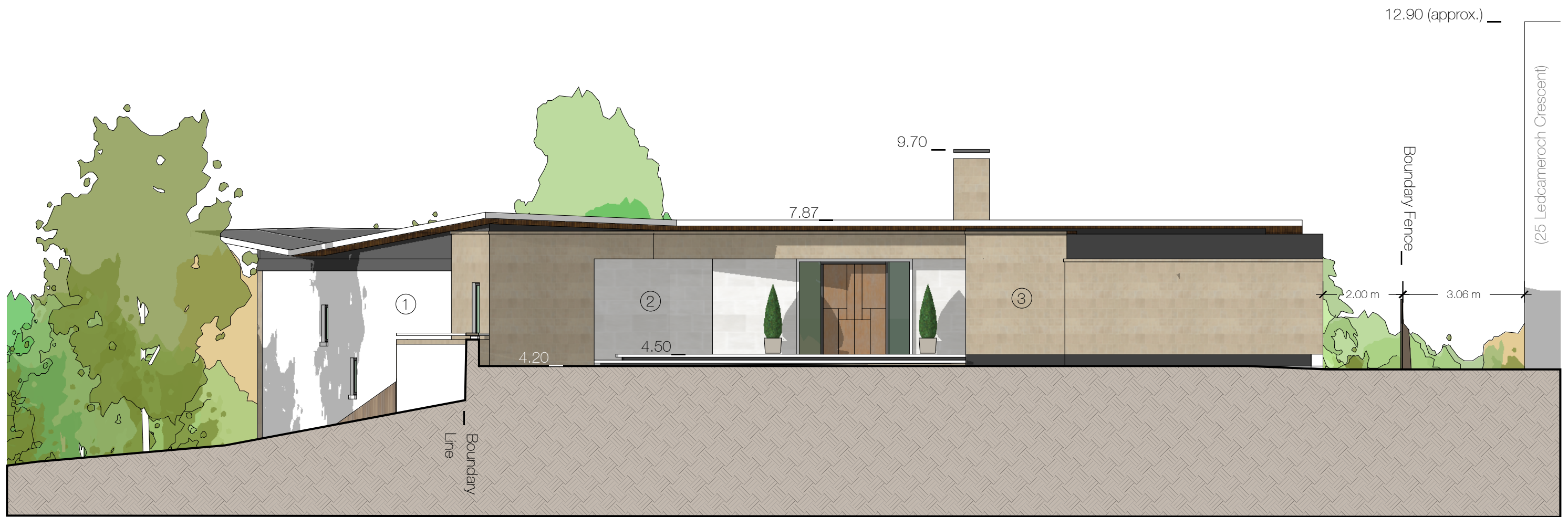
NORTH EAST ELEVATION AS PROPOSED 1:100 @ A3
