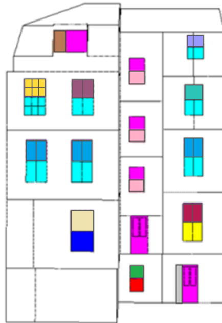
Figure 8.1.3: 10-12 Cave Street Opening Types: Back View.
