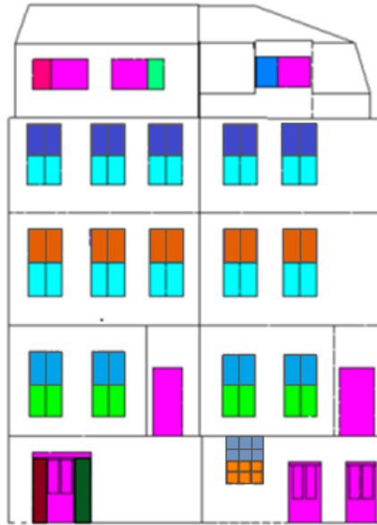
Figure 8.1.1: 10-12 Cave Street Opening Types – Front View.
