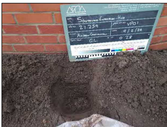
Photograph 3 - VP01, soil depth of 0.28 m. Geotextile visible at the base.
