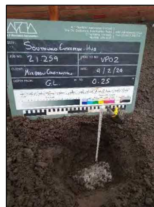
Photograph 4 - VP02, soil depth of 0.25 m. Geotextile visible at the base.
