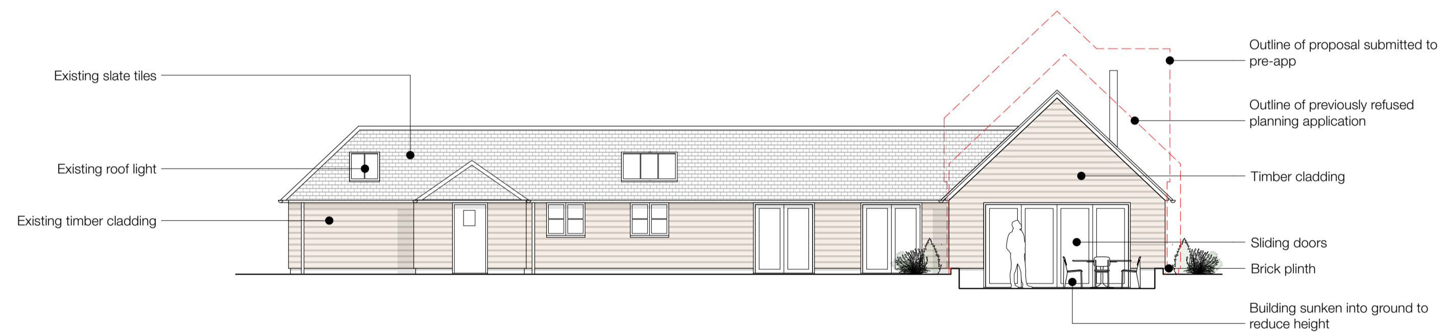
3 PROPOSED REAR ELEVATION Scale 1:100
