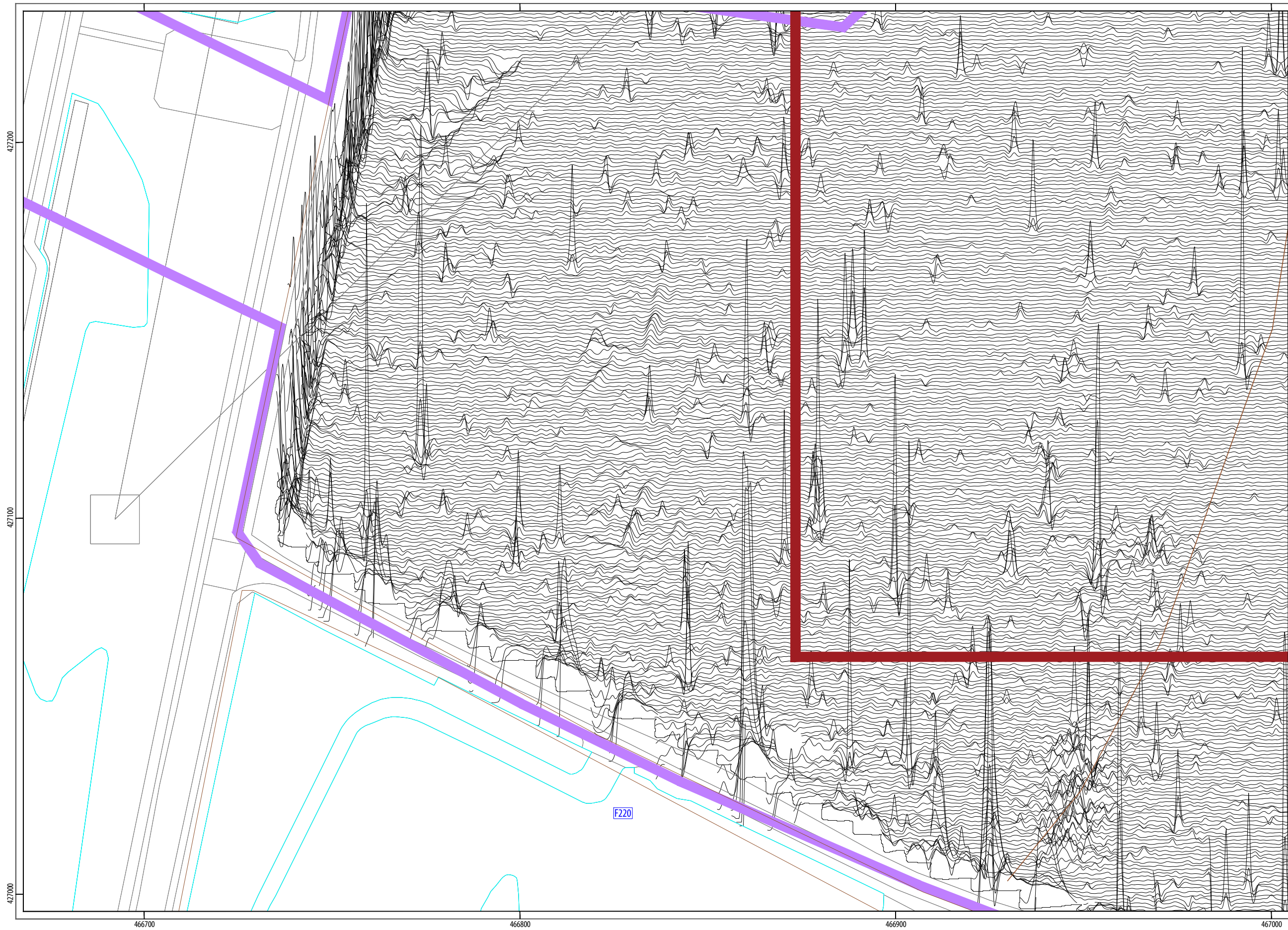
ILLUS 322 XY trace plot of minimally processed magnetometer data; AAA16
