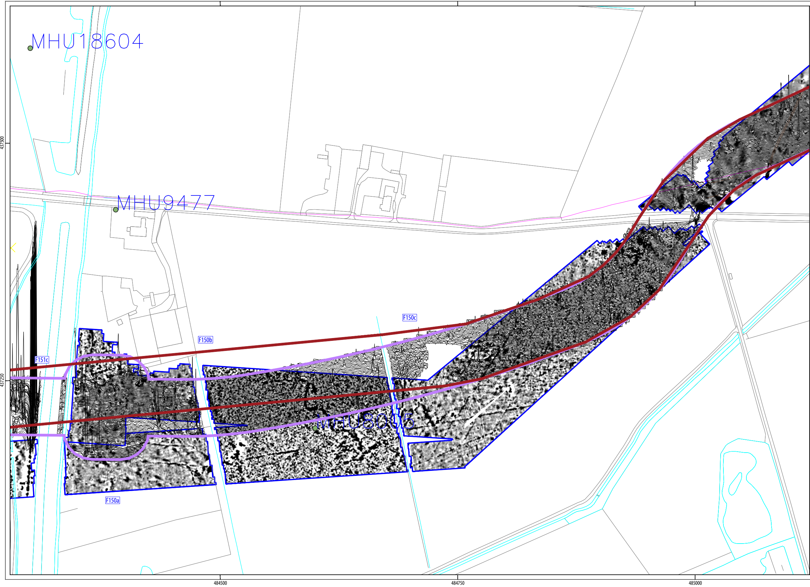
ILLUS 199 XY trace plot of minimally processed magnetometer data; Sector 53
