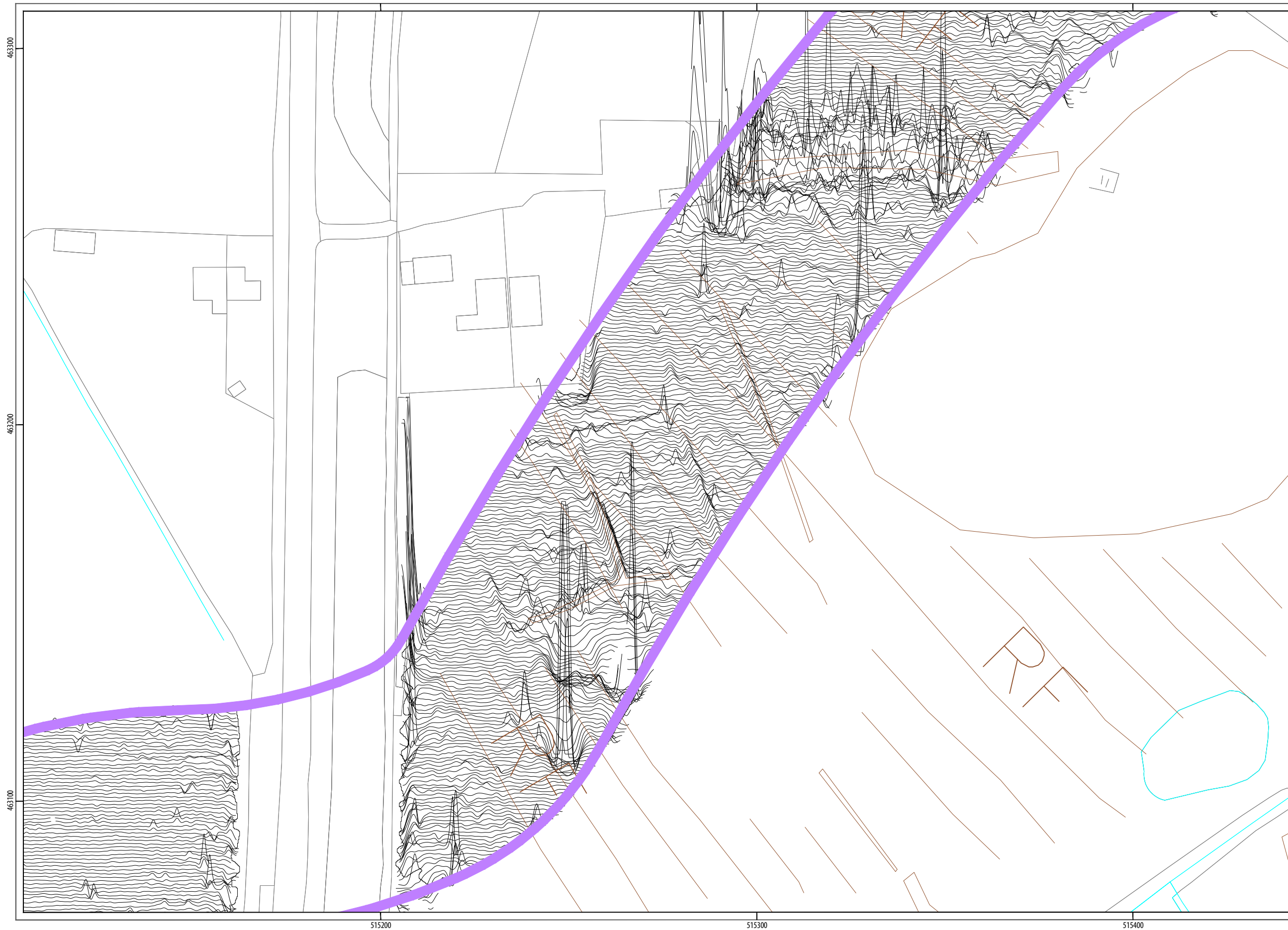
ILLUS 280 XY trace plot of minimally processed magnetometer data; AAA2
